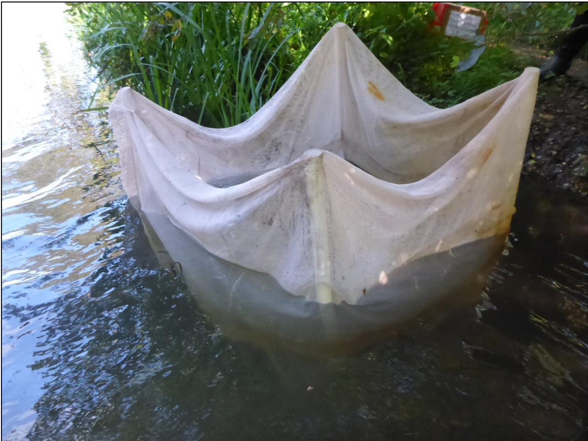
Figure 2.1. The 1 m 2 lamprey survey quadrat in situ on the River Itchen.
